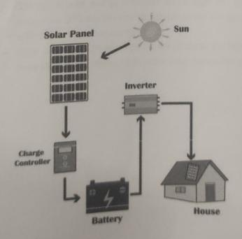
**Uses of Panel:** - Energy from the sun referred to as solar energy, is captured by the solar panels and is then converted into electricity. The solar panel is composed of many solar cells.
